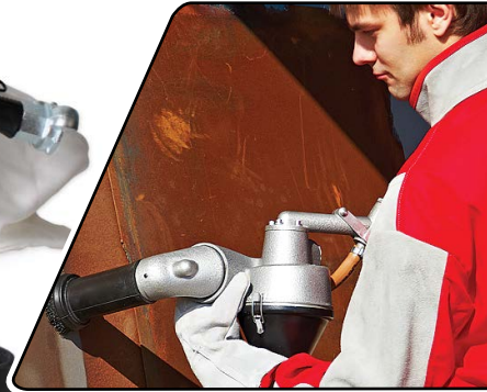
Hand-portable closed-circuit blast tool.
