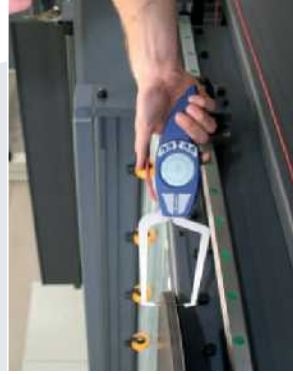
▶ Measuring calipers option: The clever tool for automatic thickness measurement.
